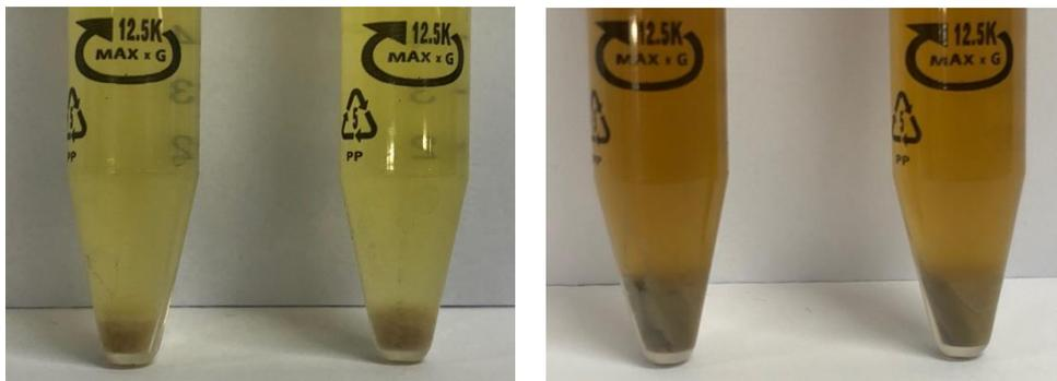
Figure 14: Separation between solid and liquid phase after centrifugation (3 minutes @ 6500 rpm) for left: pure urine (I) and right: contaminated urine (II).
