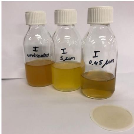
Figure 22: Fraction I: Pure urine: untreated, 0.5 µm prefiltered and 0.45 µm SDI permeate and the fouling layer on the membrane used for SDI determination.
